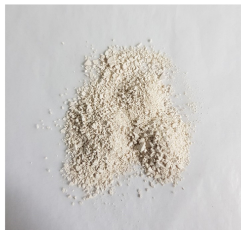
Figure 1. Digital photograph of as-prepared polyurea-based POP (UPOP) synthesized by condensation between melamine and 1,4-phenylene diisocyanate.
