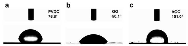
Figure 5. Contact angle of water on (a) PVDC; (b) GO; (c) AGO film.
