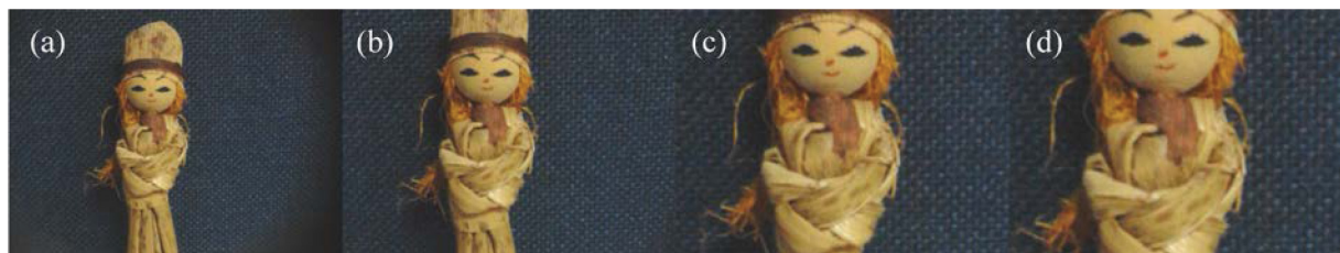
Figure 8. Images acquired under different displacement loads, from (a) to (d), the displacement load \Delta L imposed to the lens surface is 0 mm, 0.5 mm, 0.75 mm, and 1 mm.
