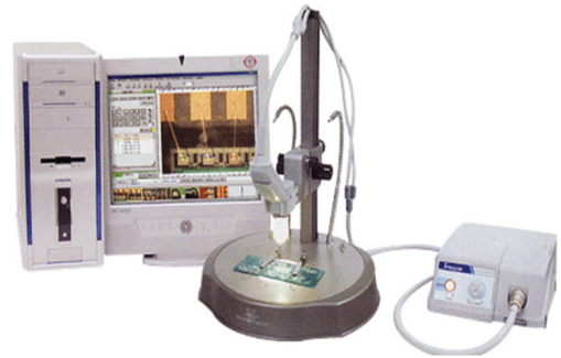
Figure 8. Image microscope used for analysis of cracks in a specimen.
