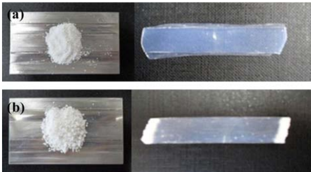
Figure 3. Photographs of dried core/PBA/PS double shell and their compressed specimens processed at 25 °C under 13.8 MPa for 5 min: (a) DS-1; (b) DS-2.
