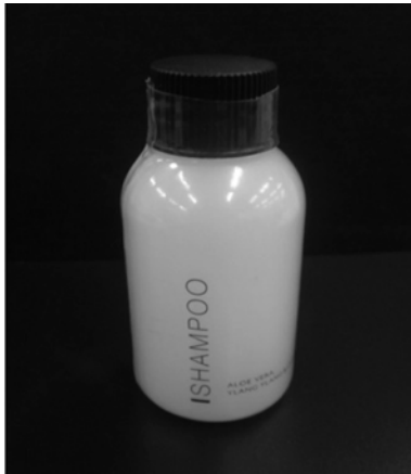
Figure 7. Picture of the bottle labeled with PLA/PPC/PLA multi-layer film in a bath at 90 °C for 10 sec.
