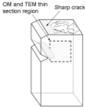
Figure 3. Schematic of the DN-4PB specimen used for OM and TEM observation.
