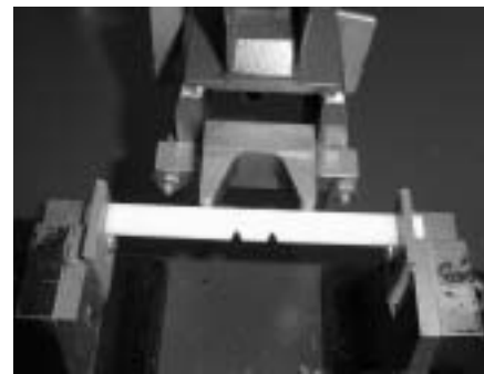
Figure 2. Geometry and fixture of the DN-4PB Charpy impact test.
