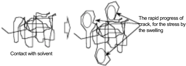
Figure 1. A mechanism of ESCR (environmental stress crack).
