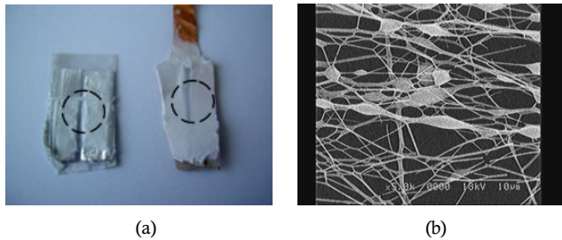
Figure 6. (a) Separated electrodes and electrospun fibers and (b) SEM micrographs of MWNT/PMMA (0.5 wt%/10 wt%) aligned nanofibers electrospun from DMF ( \times 5000 ).
