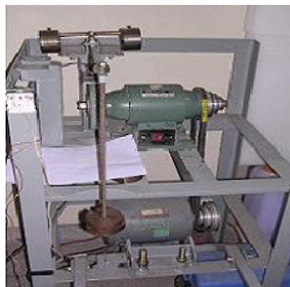
Figure 2. Picture of pin on disk type wear tester.
