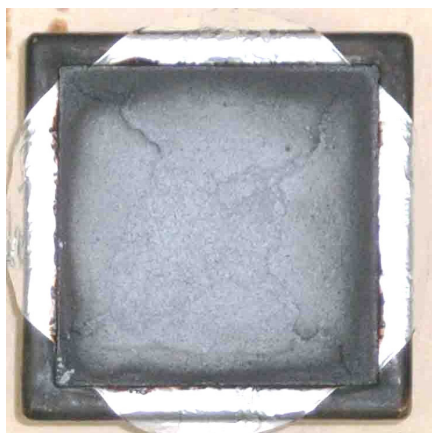
Figure 16. Char formation of the NBR/GTR compounds (specimen 3).
