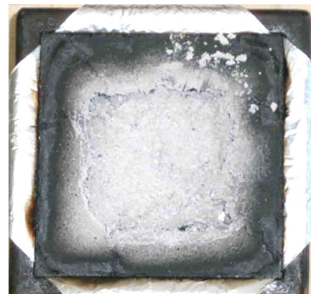
Figure 17. Char formation of the NBR/GTR compounds (specimen 5).
