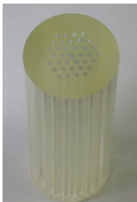
Figure 1. A preform of fabricated polymer photonic crystal fibers.
