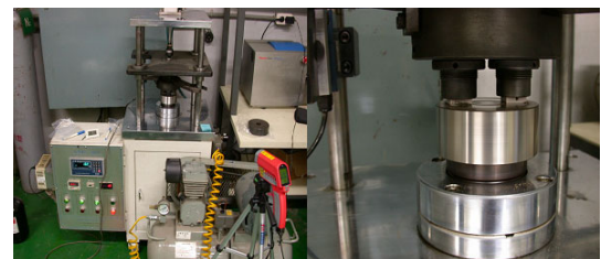
Figure 2. Photographs of wear test machine.
