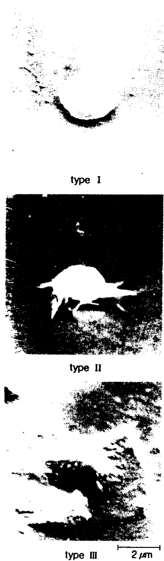
Figure 11. Scanning electron micrographs of adhered and deformed platelets on the surface of segmented polyurethane.
