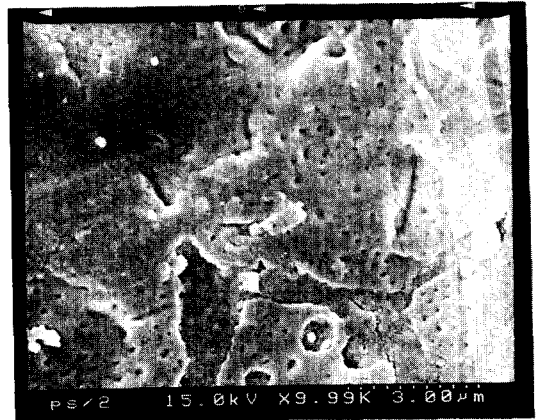
Figure 7. A photograph of scanning electron microscopy of the calcium carbonate encapsulated by polystyrene.
