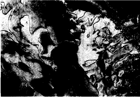
Figure 2. Photomicrograph of LCP taken at 260°C (Magnification 200×).
