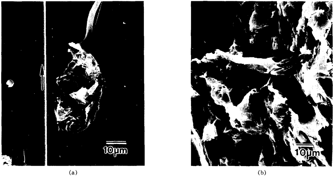
Fig. 9. Scanning electron micrographs of fracture surface of modified DGEBA epoxy showing (a) crack bifurcation and crack bridging mechanisms (Arrows indicate the crack propagation direction) (b) ductile fracture of cellulose particles.
