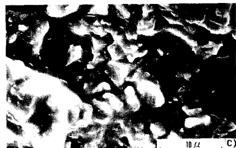
Fig. 2. Scanning electron micrographs of the master batches prepared under (a) nitrogen, (b) air, and (c) oxygen atmosphere.
