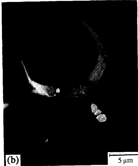
Fig. 6-(a),(b). Transmission electron micrograph showing cracks around PS domain in PAr/PS(70/30) alloy.
