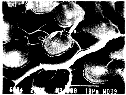
Fig. 11. Fracture surface of OXI-PAN C/C composites carbonized at 1300°C.
