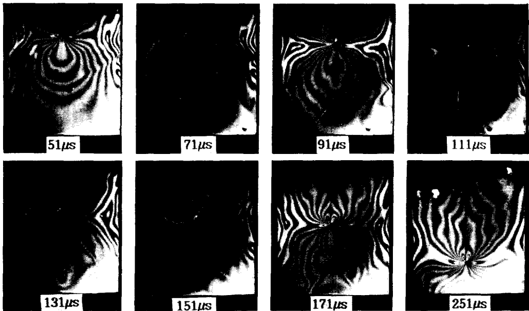
Fig. 3(a). Dynamic isochromatics in 6mm thick polycarbonate WL-RDCB specimen.
