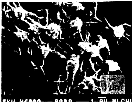
Fig.6. Scanning electron micrographs of appearances of the adhered platelet on the PMLG homopolymer surface.
