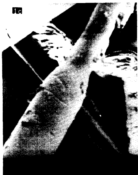
Fig. 7. Scanning electron micrograph of gel-spun filament drawn at 25°C for 4 times. The magnification is \times 610 . Necking is visible.
