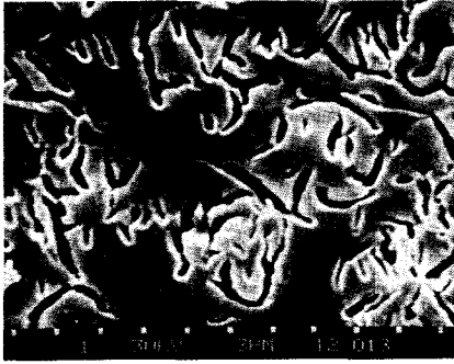
Fig. 11. SEM of cross-section of oxidized PAN fibre / phenolic resin composite, HTT 1000°C.
