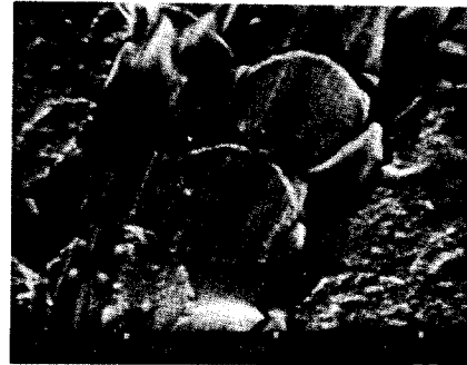
Fig. 10. SEM of cross-section of oxidized PAN fibre / phenolic resin composite, HTT 800°C.
