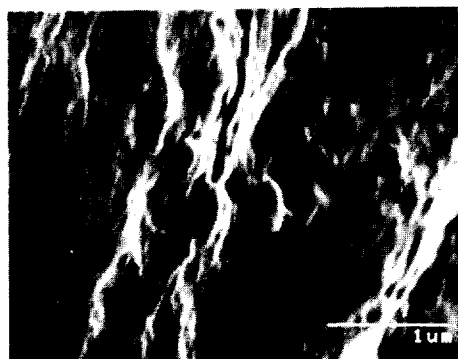
Fig. 16. Scanning electron micrograph for carbon black (ISAF) 50 phr and oil 10 phr loaded TOR Vulcanizate. Magnification: \times 30,000 .
