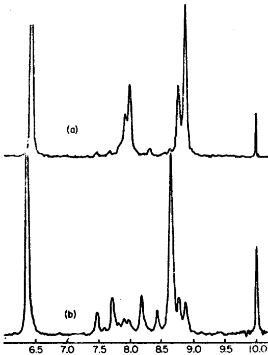
Fig. 2. The 60 MHz spectra of 15% (w/v) solutions in chlorobenzene of polymethyl methacrylate prepared with (a) a free-radical initiator and (b) an anionic initiator (PhMgBr). The ester methyl resonance appears near 6.5 \tau , the \beta -methylene protons appear near 8.0 \tau and the \beta -methyl protons give three peaks between 8.5 and 9.0 \tau .
