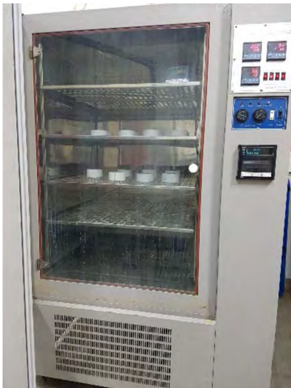
Fig. 2. Accelerated carbonation test setup.
