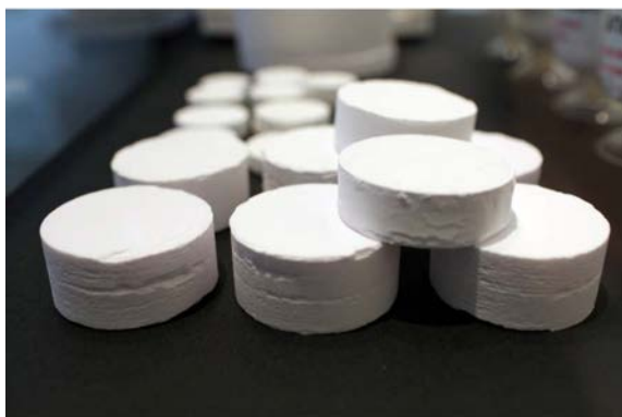
Fig. 9. Photograph of fired high-purity, high-density alumina samples.
