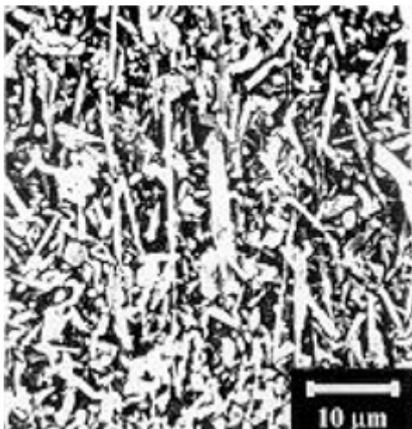
Fig. 4. SEM micrograph of structure inside Si 3 N 4 cells of Si 3 N 4 fibrous monolithic ceramic.
